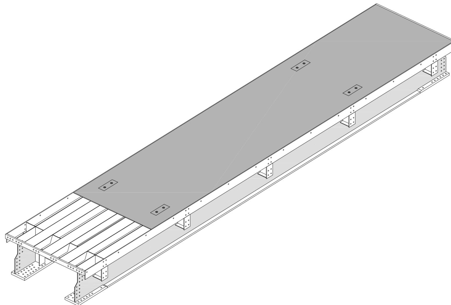
SCHEMA ASSONOMETRICO TIPOLOGICO DI UN SINGOLO MODULO DELL'IMPALCATO STRADALE
